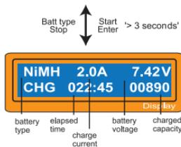
impedance and small capacity can lead to the higher charge current by the processor at automatic charge mode. But in 'Man' mode, it will charge the battery with the charge current you set at the display. Each mode can be switched by pressing INC and DEC button simultaneously when the current field is blinking.
