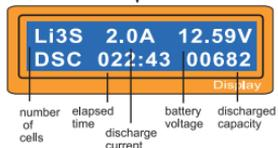
This shows the present state of discharge. To stop discharging press Batt type/Stop key once.
