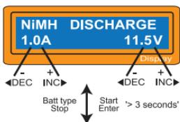
Set discharge current on the left and final voltage on the right. The discharge current ranges from 0.1 to 5.0A and the final voltage ranges from 0.1 to 30.0V). To start the process, press Start /Enter key for more than 3 seconds.
