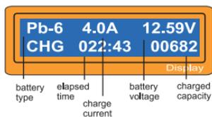
The screen displays the state of charging process. To stop charging forcibly, press Batt type/Stop key once. The audible sound indicates you at the end of process.
