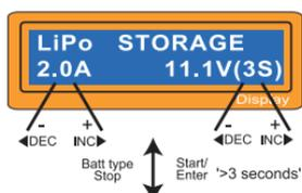
You can set up the current and the voltage of the battery pack to be charged. The current will be used for charge or discharge the battery to reach the 'storage' level of voltage.
