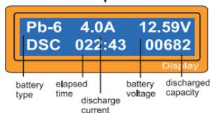
Set discharge current on the left and final voltage on the right. The discharge current ranges from 0.1 to 5.0A.
