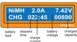
The screen displays the current state of discharge. You can alter the discharge current by pressing Start/Enter key during the process. Once you change the current value, store it by pressing Start /Enter button again.
