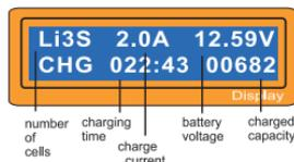
After setting the current and voltage press Start/Enter key for more than 3 seconds to start the process.
