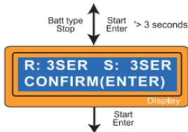
This shows the number of cells you set up and the processor detects. 'R:' shows the number of cells found by the charger and 'S:' is the number of cells selected by you at the previous screen. If both numbers are identical you can start charging by press Start/Enter button. If not, press Batt type/Stop button to go back to previous screen. Then carefully check the number of cells of the battery pack to charge again.
