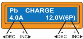
Set up the charge current on the left and the nominal voltage of the battery on the right. The charge current ranges from 0.1 to 7.0A and the voltage should be matched with the battery being charged. Start the charge process by pressing Start/Enter key for more than 3 seconds.
