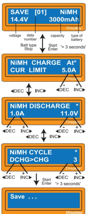
with the battery type you set up. The example shows the battery pack of NiMH, 12cells and 3000mAh of capacity.
