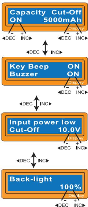
This program sets the maximum charge capacity that will be supplied to the battery during charge. If the delta-pack voltage is not detected nor the safety timer expired by any reason, this feature will automatically stop the process at the selected capacity value.
