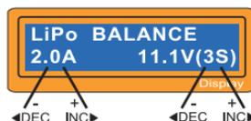
The value on the left side of second line sets a charge current and the value on the right side of second line sets the voltage of the battery pack.
