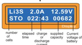
The screen shows the present situation during charge process. To stop charging press Batt type/Stop key once.
