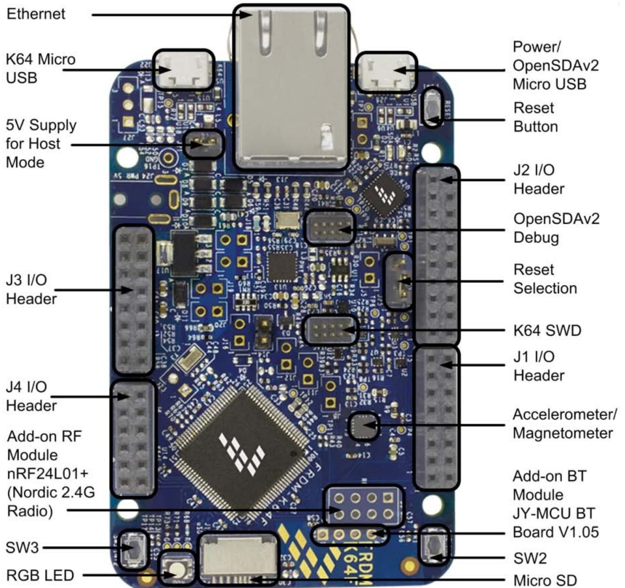
Figure 2. FRDM-K64F main components placement
