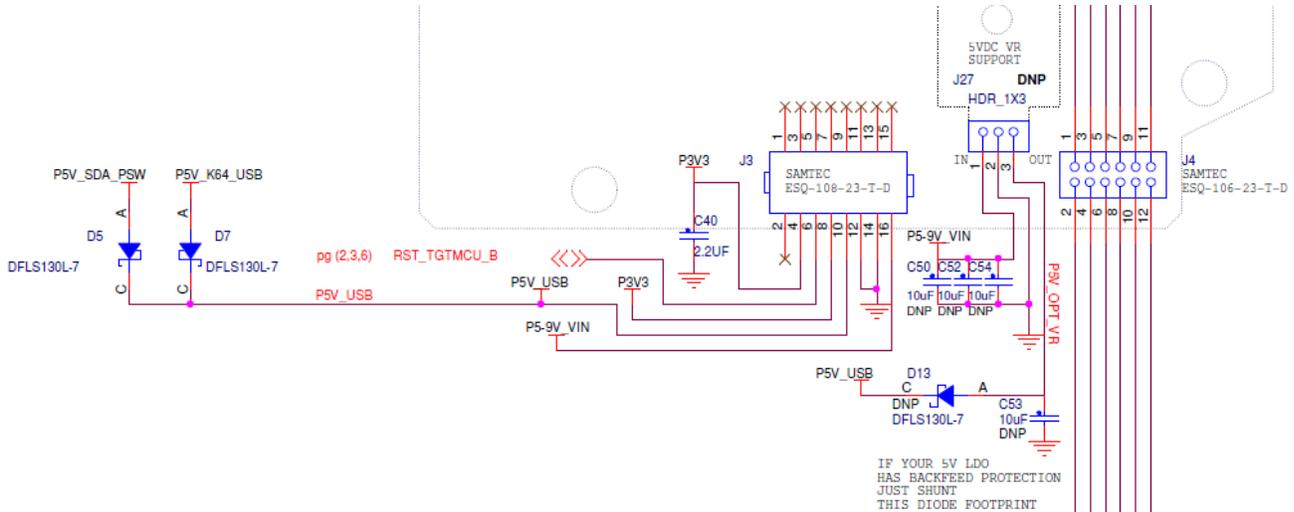
Figure 10. K64 USB power input for host mode
